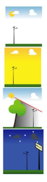
The battery gets loaded during daytime with the electricity produced by the solar panel (PV).
